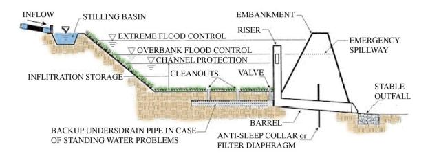
Figure 2. Cross section schematic of infiltration basin
