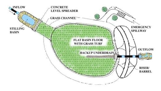
Figure 1. Schematic design of infiltration basin with concrete level spreader
