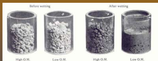
FIGURE 4.17 The aggregates of soils high in organic matter are much more stable than are those low in this constituent. The low organic matter soil aggregates fall apart when they are wetted; those high in organic matter maintain their stability.
